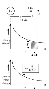
Work done w is for unit +ve test charge and is called electric potential.
