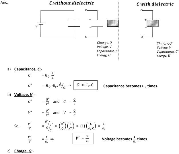
As circuit is open, charge cannot flow in the loop.
