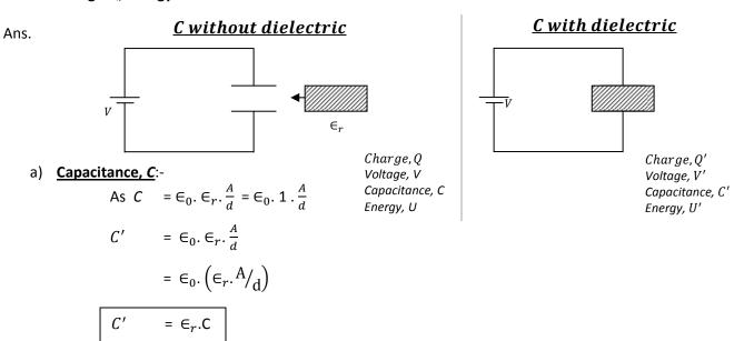
Capacitance becomes  $\in_r$  times after inserting the slab.
